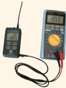
Example of 98077 output cable for screw terminal connecting to XL series data logger
