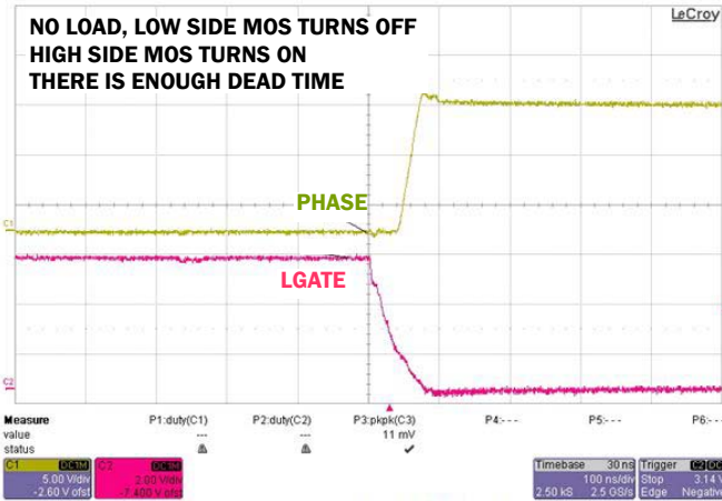
FIGURE 19. GATE DRIVER AND SWITCHING TRANSIENT
