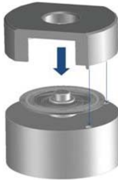
Figure 6. Set the two height tool guide pins into the two mounting holes
