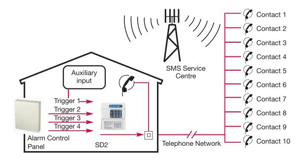
The SD2 is the ideal solution for monitoring a wide variety of processes and equipment such as temperature control, machinery, medical cabinets, vending machine stock levels, burglar and fire alarms, as well as letting you listen in and talk back to the location.
