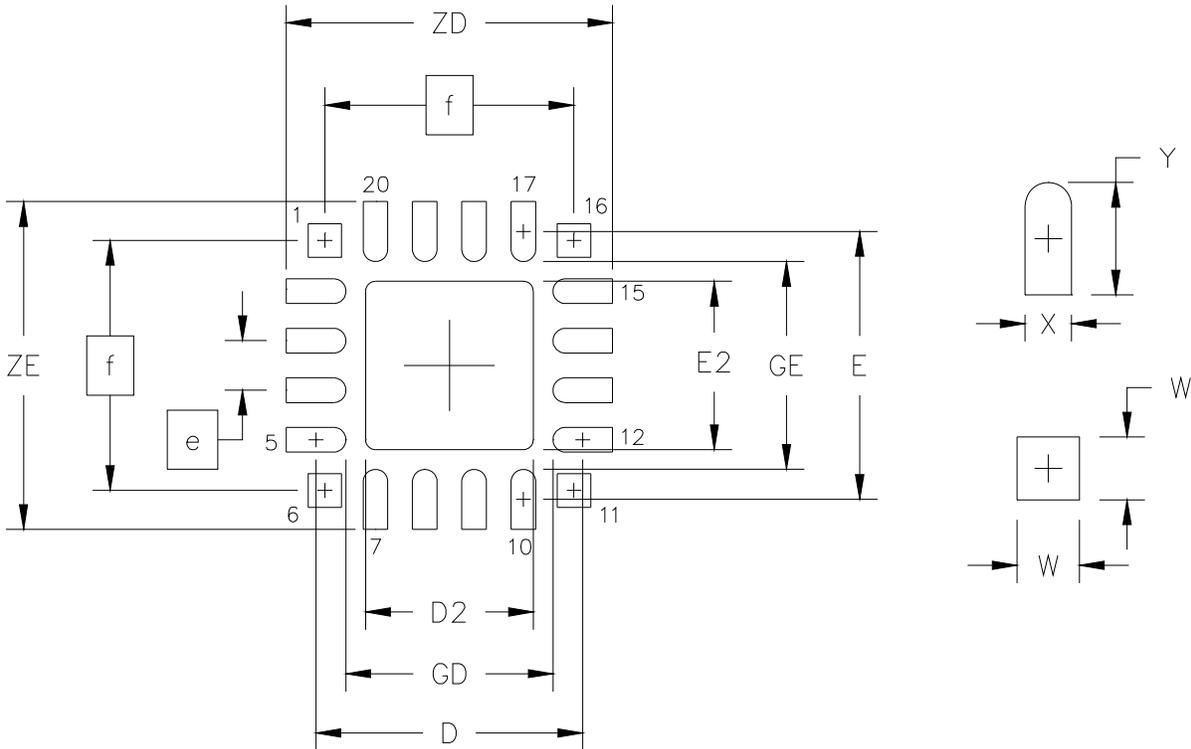
Figure 7.2. QFN-20 Landing Diagram
