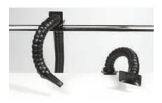
The **Omniflex Arms** (Ø63mm) are designed for higher airflow rates and effective fume capture from greater distances. A unique ball/socket design provides an unmatched flexibility in maneouvering and positioning. The arms can be adjusted in working length or radius, simply by adding or removing Omniflex components. ESD conformance is ensured through the use of fully conductive material.
