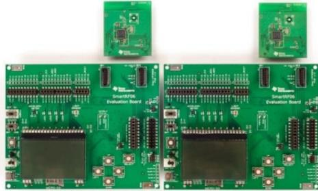
2 x SmartRF06 Evaluation Boards (SRF06EB)
