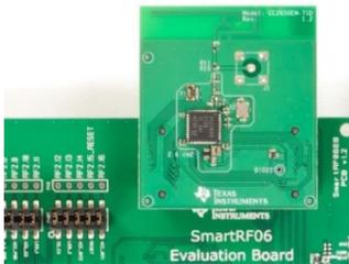
Insert a CC2650EM board into the SmartRF06EB as shown above.
