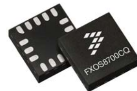
16 LEAD QFN 3 mm x 3 mm x 1.2 mm
