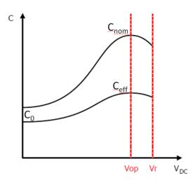
Initial capacitance C<sub>0</sub>: is the value at the origin of the hysteresis without any applied direct
