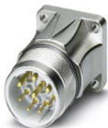
Device connector, front mounting, straight, Screw locking, M23, Number of positions: 4+3+PE, Type of contact: Male connector, Crimp connection, Axial O-ring, 4xØ3,2, shielded: Yes, Flange dimensions: 26 mm x 26 mm, Cable diameter: 0 mm...0 mm, Compatible with mating connectors with SPEEDCON or M23 standard knurled nuts
