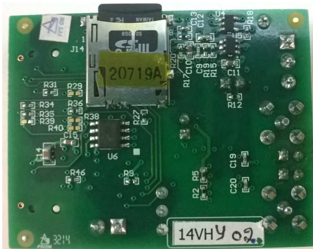
Figure 4. Bottom View of ADS7043EVM Board with microSD Memory Card Installed
