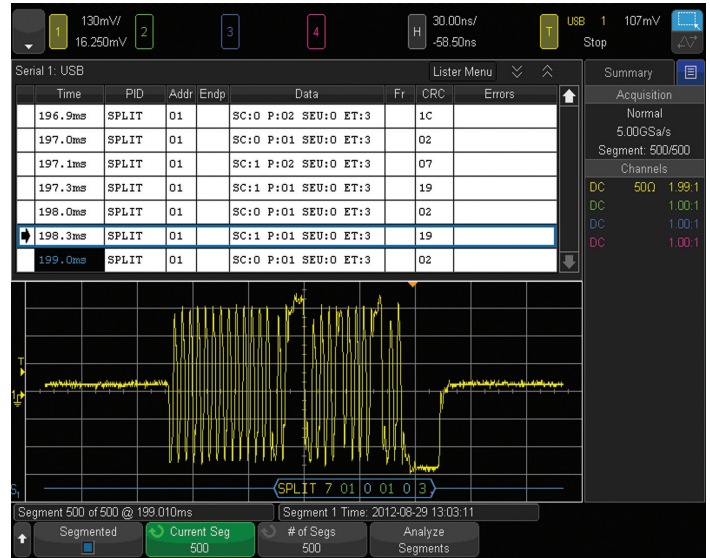
Figure 5: Segmented memory acquisition selectively captures more packets/bytes of serial bus activity.
