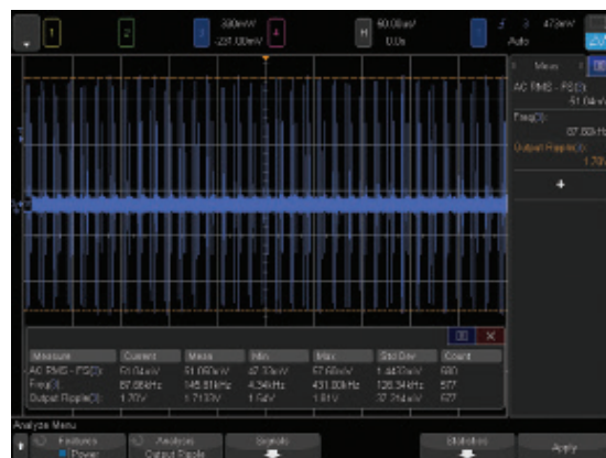
Figure 6. The output analysis includes characterizing the ripple component (either power line or switching) in output DC voltage.
