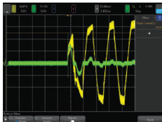
Figure 3. The inrush current analysis measures the peak inrush current of the power supply when the power supply is first turned on.
