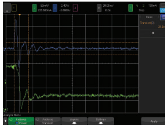
Figure 8. The transient analysis measures the load transient response of the DC output, namely the time taken for the DC output to stabilize during a load change.
