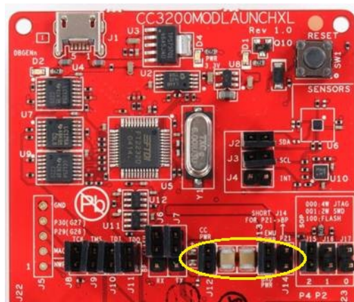
Figure 9. Powering From USB
