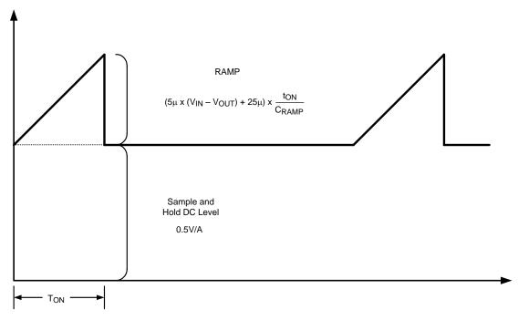
Figure 14. Composition of Current Sense Signal
