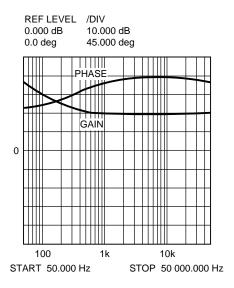
Figure 18. Error Amplifier Gain and Phase
