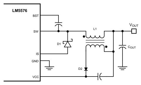
Figure 21. VCC Bias with Additional Winding on the Output Inductor
