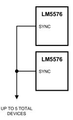
Figure 11. Sync from External Clock
