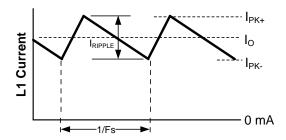
Figure 16. Inductor Current Waveform
