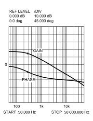
Figure 17. Gain and Phase of Modulator  $R_{LOAD} = 5$  Ohms and  $C_{OUT} = 177 \mu F$
