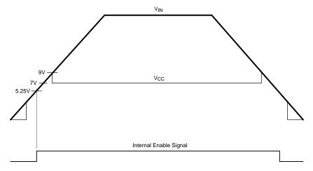
Figure 10. Vin and Vcc Sequencing
