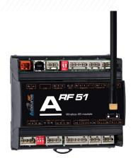
The ARF51 module is a 4 I/O (input/output) AON (All Or Nothing) acquiring data coming from sensors, contacts, or meters to control remote equipment.
