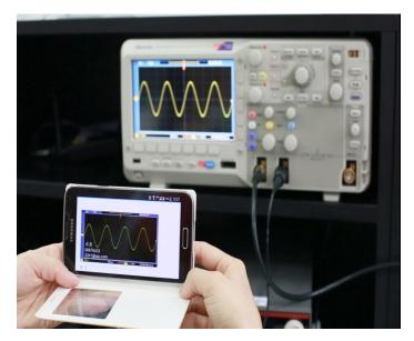
The test results, which include snapshots of the oscilloscope with step number, instruments' S/N, student's name and comments, can be downloaded locally, or archived on the lab server for future access.
