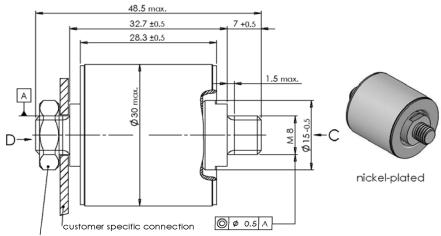
max. torque = 8 Nm counter-hold with 13mm wrench to minimize torque charge
