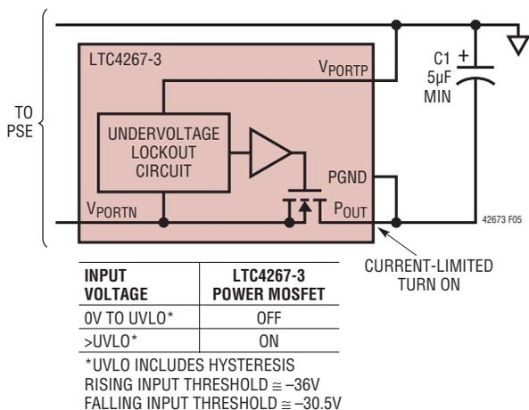
Figure 5. LTC4267-3 V<sub>PORTN</sub> Undervoltage Lockout
