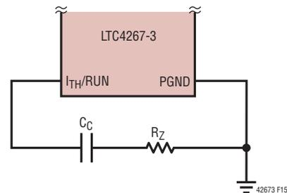
**Figure 15. Main Loop Compensation for a Nonisolated Design**
