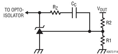
**Figure 14. Main Loop Compensation for an Isolated Design**
