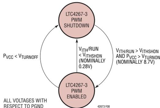
Figure 8. LTC4267-3 Switching Regulator Start-Up/Shutdown State Diagram
