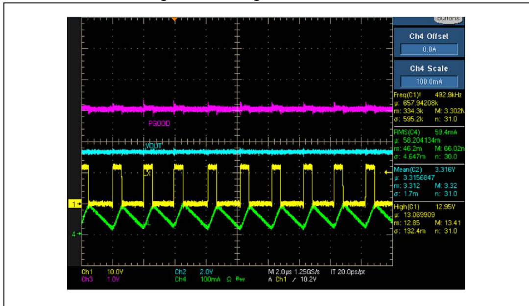
Figure 12. The regulator works in CCM
