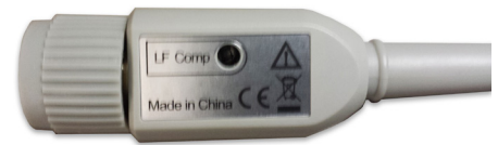
Figure 2. Low-frequency compensation adjustment (for N2840A/41A/42A/43A/53A)
