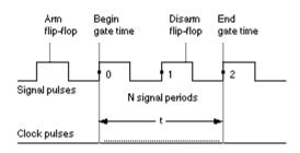
The **P6000A** measures frequency or period by counting the number of 11.059 MHz clock pulses during an actual gate time t, which corresponds to an intergral number of signal periods N. This technique allows high-accuracy low-frequency measurements. Frequency is calculated from N/t, period from t/N.
