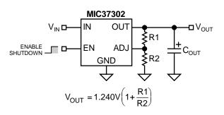
Figure 1. Adjustable Regulator with Resistors
