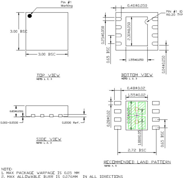
1. MAX PACKAGE WARPAGE IS 0.05 MM 2. MAX ALLOWABLE BURR IS 0.076MM IN ALL DIRECTIONS 3. PIN #1 IS ON TOP WILL BE LASER MARKED 4. RED CIRCLE IN LAND PATTERN INDICATE THERMAL VIA. SIZE SHOULD BE 0.30-0.3M IN DIAMETER AND SHOULD BE CONNECTED TO GND FOR MAX THERMAL PERFORMANCE 5. GREEN RECTANGLES (SHADED AREA) INDICATE SOLDER STENCIL OPENING ON EXPOSED PAD AREA, SIZE SHOULD BE 0.50×0.95 MM IN SIZE, 0.20 MM SPACING.
