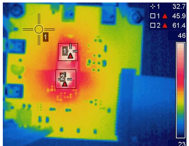
Figure 19: Thermal Image at V_{IN} = 16V , I_{OUT} = 6A (IR3863: 61°C, Inductor: 46°C, PCB: 33°C)
