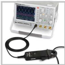
This AC/DC current probe is used to measure currents from 1mA to 30A over a broad frequency range. The measurement principle is based on the Hall Effect that registers the magnetic field generated by the current flow. Even for complex waveforms a high degree of measurement accuracy is achieved. The output voltage is proportional to the measured current and well suited to be displayed on an oscilloscope. The current probe complies with the safety standards defined in IEC/EN 61010.
