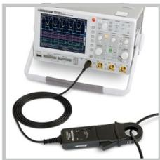
This AC/DC current probe is used to measure currents from 100mA to 1000A over a broad frequency range. The measurement principle is based on the Hall Effect that registers the magnetic field generated by the current flow. Even for complex waveforms a high degree of measurement accuracy is achieved. The output voltage is proportional to the measured current and well suited to be displayed on an oscilloscope. The current probe complies with the safety standards defined in IEC/EN 61010.
