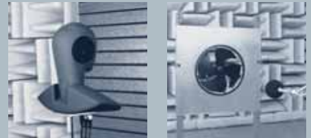
Room for precision noise measuring
