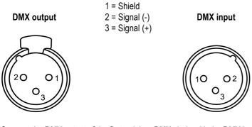
Connect the DMX output of the first unit in a DMX chain with the DMX input of the next unit in the chain. Always connect the the output of one unit with the input of the next unit until all units are connected.
