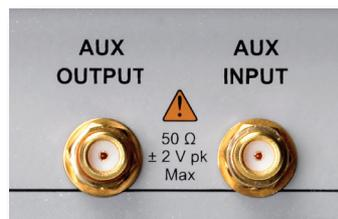
These can be used to test the instrument's inputs, experiment with its features and verify complex setups such as mask tests. AUX OUTPUT can also be configured as a trigger output.
