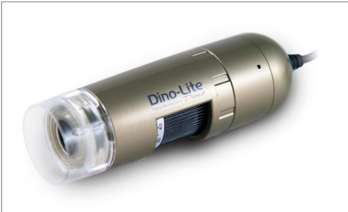
By using a special polarization filter, the AD4113ZT is the right choice when working with high glare materials such as plastics and metals. This model is delivered with three exchangeable caps: an open cap, a closed cap and a cap with polarization filter.
