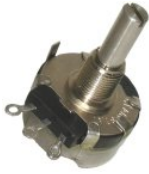
RV4 Series Industrial Potentiometer, Conductive Plastic Element, Solder lug Terminals, 2 W Power Rating, 1 kOhm Resistance Value
