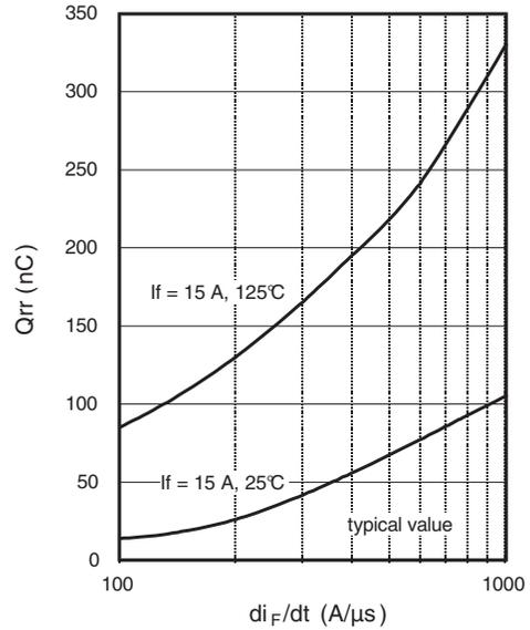
Fig. 10 - Typical Stored Charge vs.  $di_F/dt$
