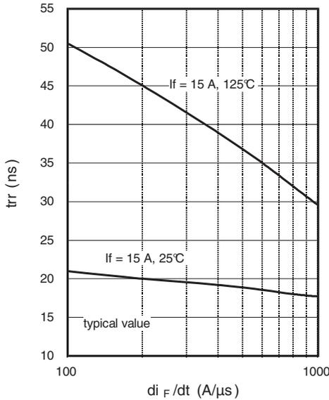
Fig. 9 - Typical Reverse Recovery vs.  $di_F/dt$
