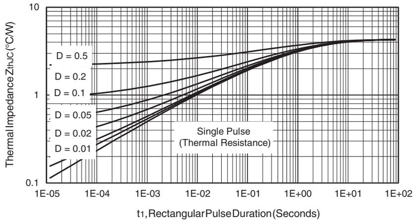
Fig. 5 - Maximum Thermal Impedance  $Z_{thJC}$  Characteristics (FULL-PAK)
