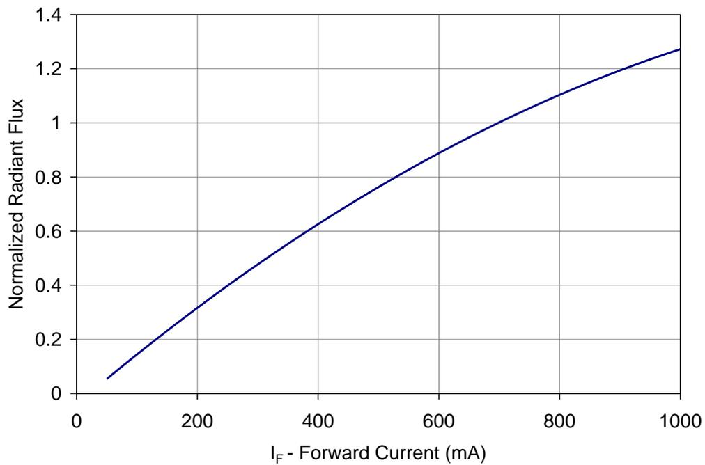
Figure 7: Typical normalized radiant flux vs. forward current @ T<sub>c</sub> = 25°C.
