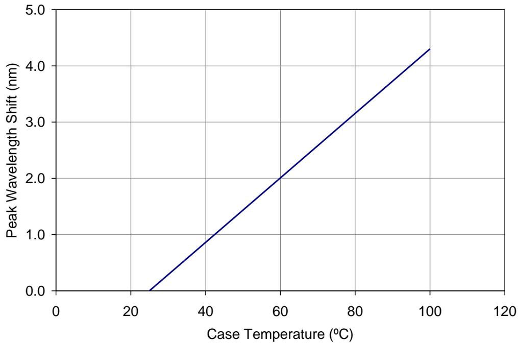
Figure 6: Typical peak wavelength shift vs. case temperature.
