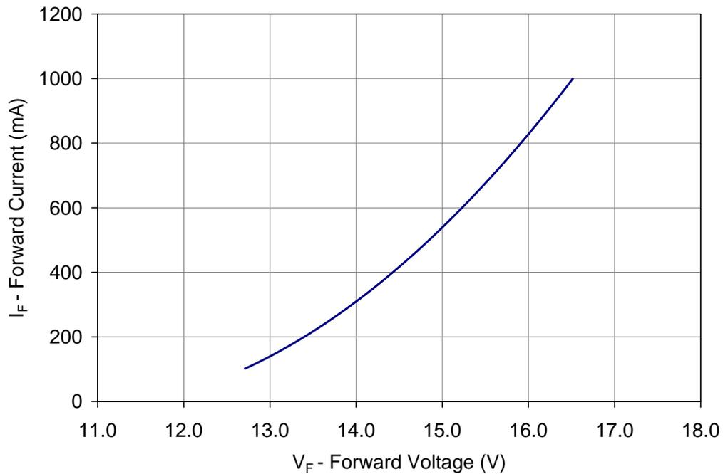
Figure 9: Typical forward current vs. forward voltage @ T<sub>C</sub> = at 25°C.
