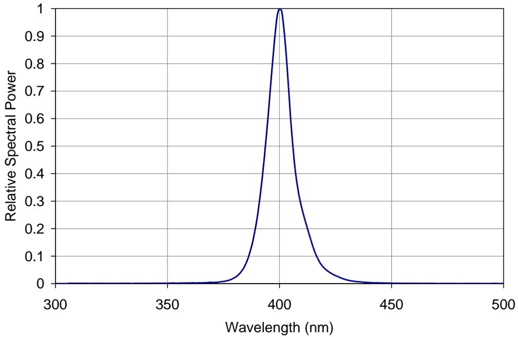
Figure 5: Typical relative spectral power vs. wavelength @ T<sub>c</sub> = 25°C.
