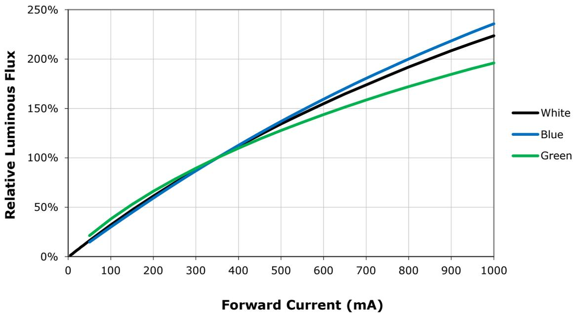
**RELATIVE FLUX VS. CURRENT ( $T_j = 25\text{ }^\circ\text{C}$ ) - CONTINUED**
