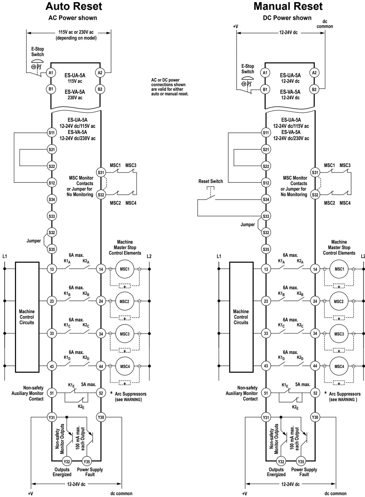
Figure 5. Wiring for 1-Channel E-Stop Applications
