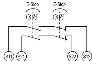
Figure 2. Series connection of multiple E-stop switches
