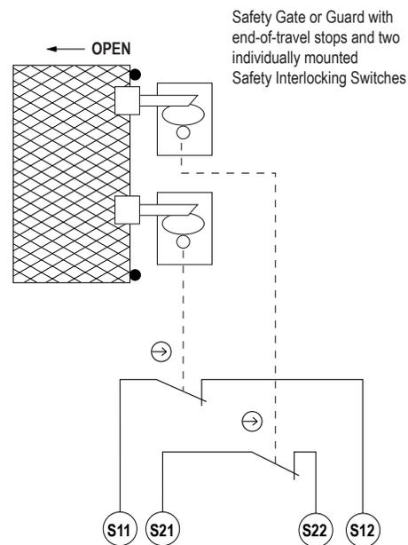
Figure 3. Wiring using contacts from two safety switches
