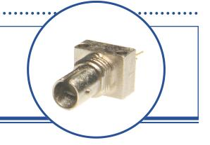
The OPF322 family fiber optic transmitters are high performance devices packaged for data communication links. This transmitter is an 850nm GaAlAs LED and is specifically designed to efficiently launch optical power into fibers ranging in size from 50/125µm up to 200/300µm diameter fiber. Multiple power ranges with upper and lower limits are offered which allows the designer to select a device best suited for the application.
