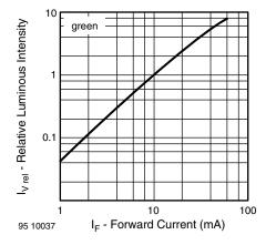
Fig. 7 - Relative Luminous Intensity vs. Forward Current
