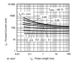
Fig. 2 - Forward Current vs. Pulse Length
