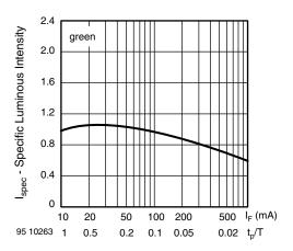
Fig. 6 - Specific Luminous Intensity vs. Forward Current
