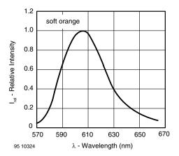
Fig. 4 - Relative Intensity vs. Wavelength
