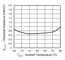
Fig. 6 - Sensitivity vs. Ambient Temperature
