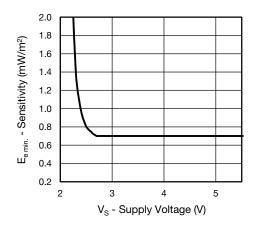
Fig. 10 - Sensitivity vs. Supply Voltage
