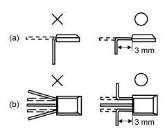
Bending position of lead wire
