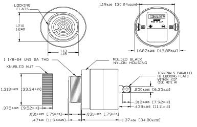
NOTE A: TERMINALS-.032 BRASS TIN PLATED, TAPPED FOR #6-32 SCREW. TWO #6-32 NICKEL PLATED BRASS SCREWS INCLUDED. WILL ACCEPT 1/4' QUICK CONNECT. NOTE B: MOUNTING- REMOVE BLACK PLASTIC NUT AND INSERT THREADED FRONT THROUGH 1.25' HOLE PUNCHED IN PANEL, IF DRIENTATION IS NEEDED, NOTE LOCKING FLATS ON DRAWING. SCREW NUT BACK ON. DO NOT OVERTIGHTEN.
