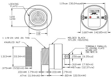
NOTE A: TERMINALS-.032 BRASS TIN PLATED, TAPPED FOR #6-32 SCREW. TWO #6-32 NICKEL PLATED BRASS SCREWS INCLUDED. WILL ACCEPT 1/4' QUICK CONNECT. NOTE B: MOUNTING- REMOVE BLACK PLASTIC NUT AND INSERT THREADED FRONT THROUGH 1.25' HOLE PUNCHED IN PANEL, IF DRIENTATION IS NEEDED, NOTE LOCKING FLATS ON DRAVING, SCREW NUT BACK ON. DO NOT OVERTIGHTEN.
