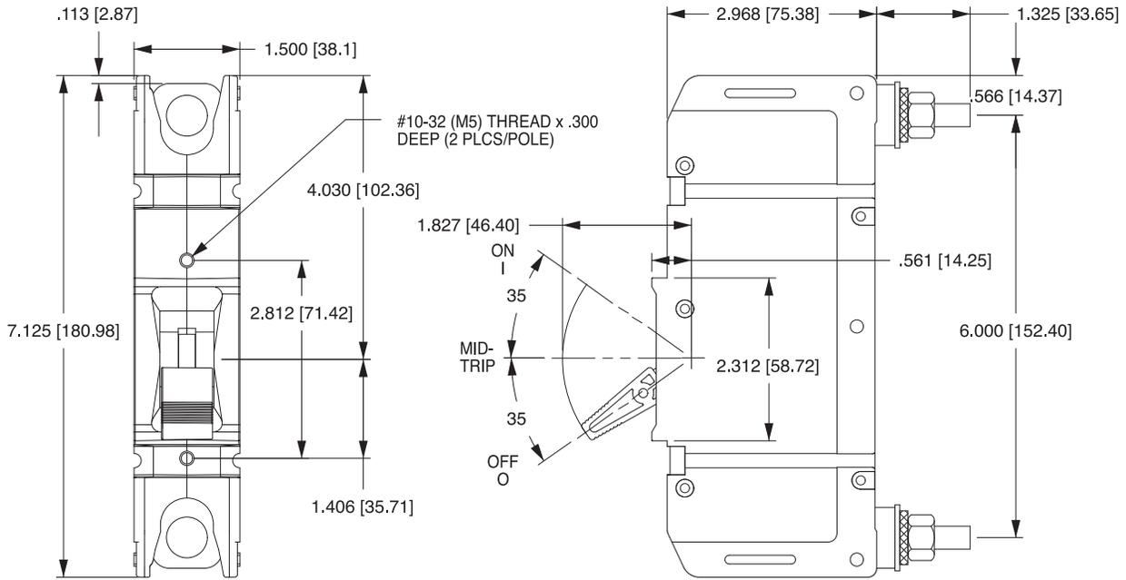
**MULTIPOLE SERIES TRIP, SHOWING TERMINAL BARRIER**
