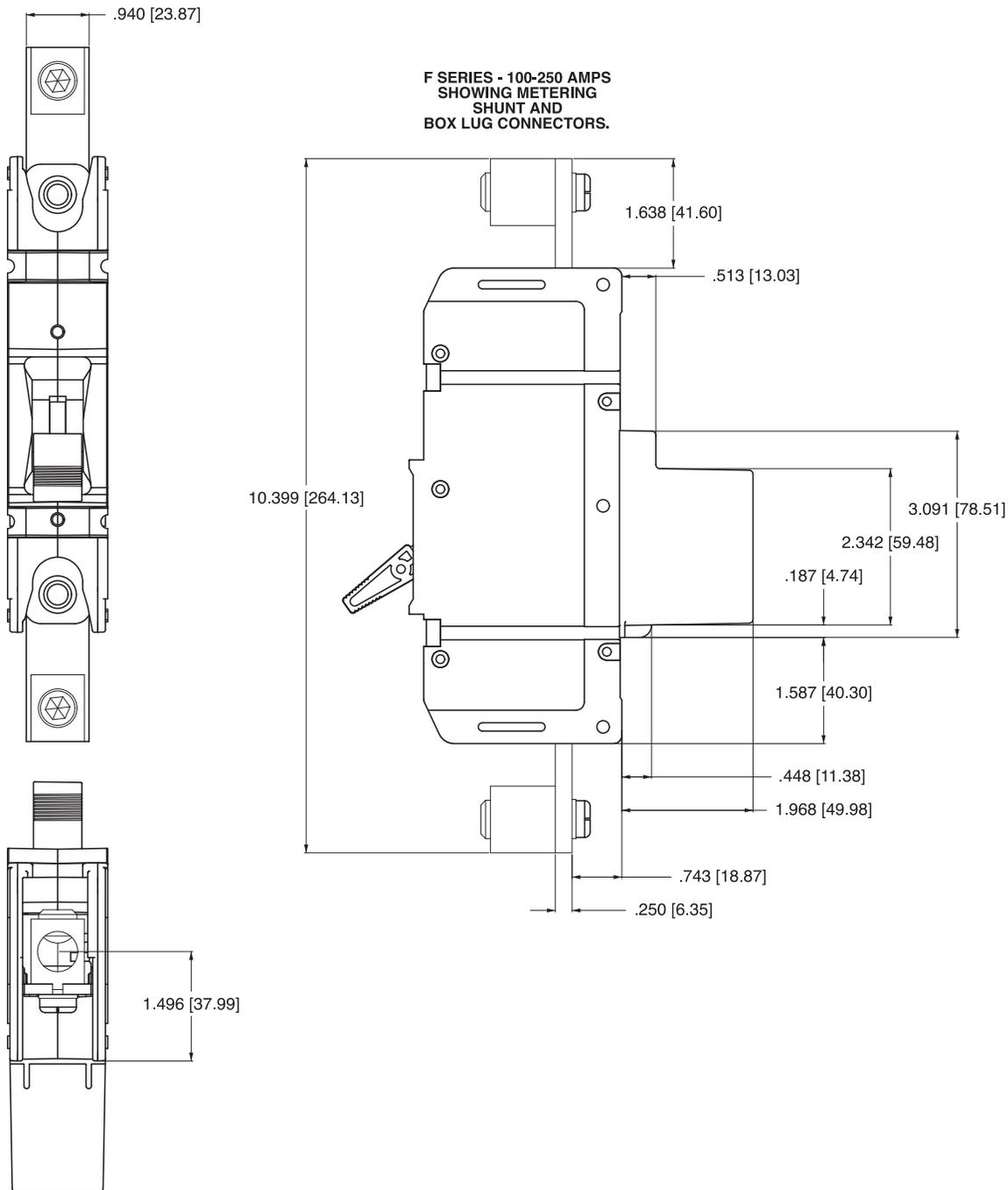
F-Series breakers are available up to 700A, and are also available with a 25 millivolt metering shunt construction. This optional construction provides a safe method for monitoring current flowing through the breaker by simply connecting a meter with light gauge wire to the appropriate terminals located on the shunt housing at the rear of the breaker. You can customize the application by measuring and displaying percentage of current, watts or safe/danger zones.
