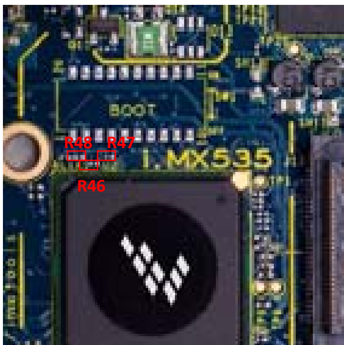
Figure 16. Boot Mode Resistor Locations TOP
