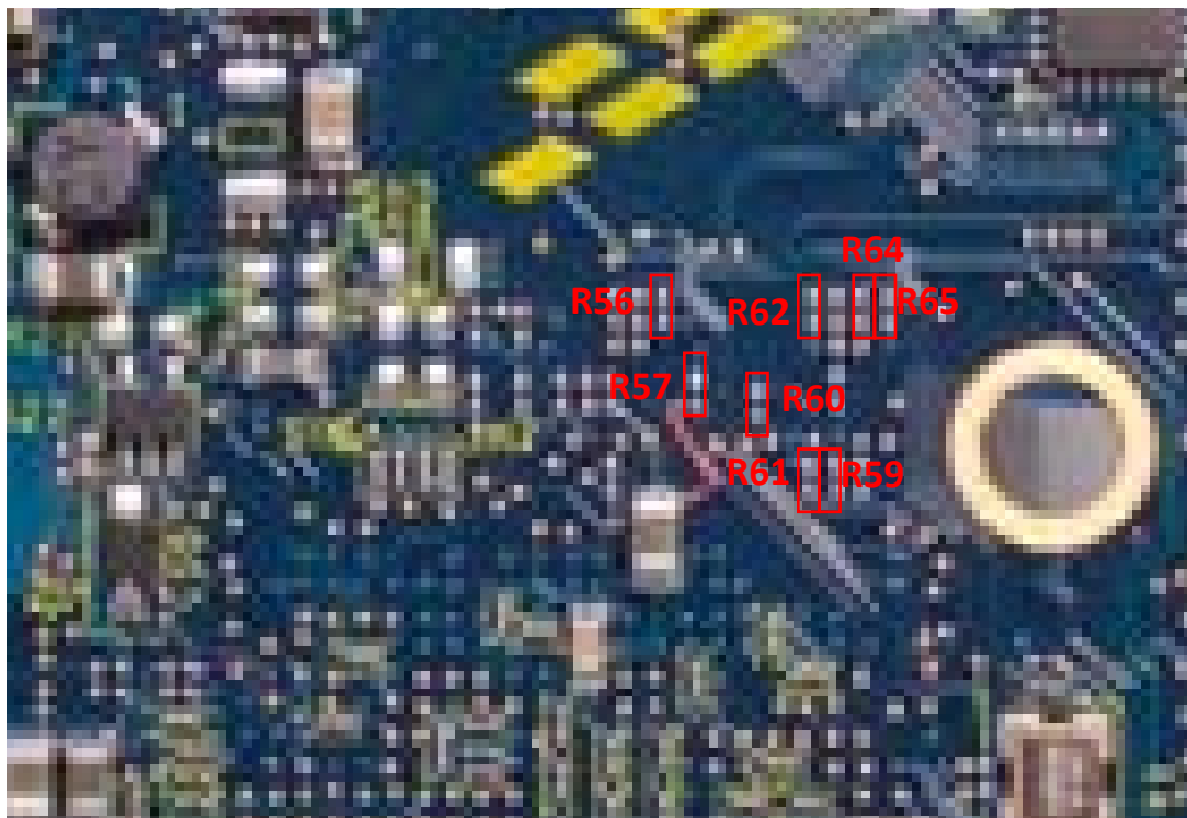
Figure 17. Boot Mode Resistor Locations BOTTOM
