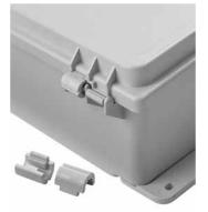
Hinge Retainers can be field-installed without modification to POLYPRO hinges for applications where easy cover removal is not desired. Two retainers per enclosure is recommended. Kit includes ten hinge retainers.
