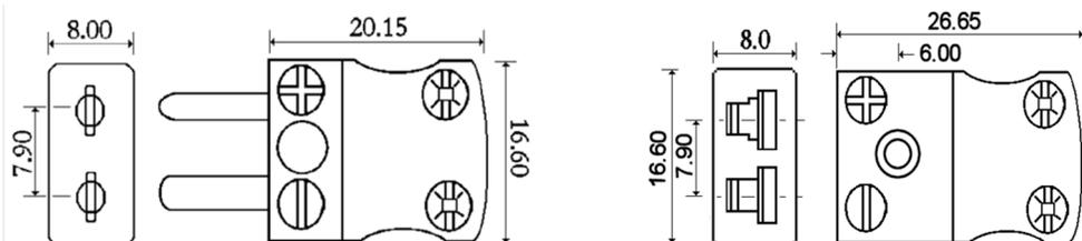
FAR015/0313. Miniature Thermocouple Plug and Socket
