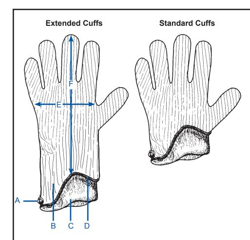
\*Glove should be grounded to verify dissipation of static charges. Use Desco 09480 coil cord or equivalent to ground.
