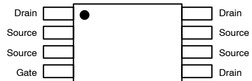
Figure 2. Pinouts for Single Die TSSOP
