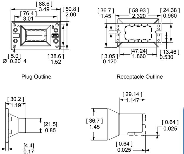
See APP's innovative MARC Connector that offers straight-on or rotational blindmate capability. MARC holds 6 PP15/45 power contacts and 2 PP15/45 premate ground contacts in a high temperature housing. Visit our website, [www.andersonpower.com](http://www.andersonpower.com) to learn more.
