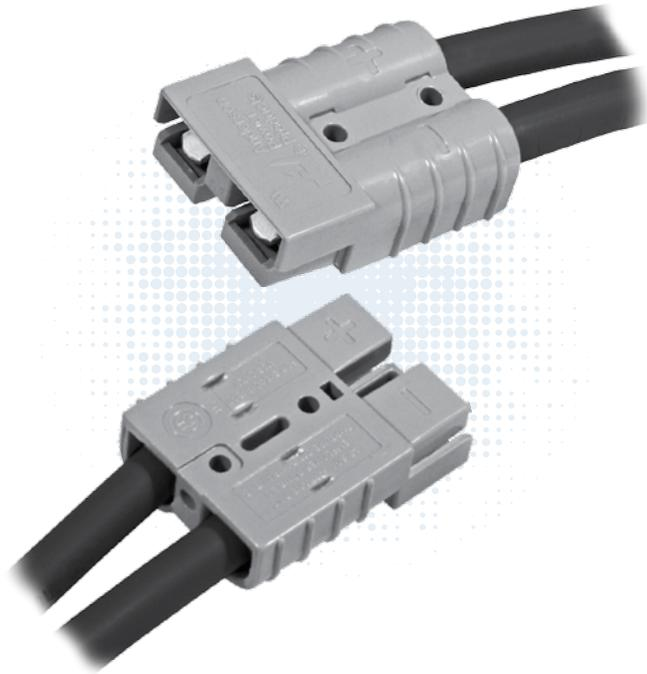
Based off the design pioneered by Anderson in 1953, APP's two pole SB® connectors set the standard for DC power distribution and battery connections. SB®50 connectors feature a one piece plastic housing using stainless steel springs to hold low resistance contacts in place. Wires sizes from #16 (1.3 mm<sup>2</sup>) to #6 (13.3 mm<sup>2</sup>) are held in the smallest of the SB® series housings.
