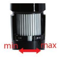
2. turn the focus knob to the far left(small magnification side), make it to be minimum; then turn the knob to the right(big magnification side) slowly and slightly, until appeared clean image under a smaller magnification, and then go on turning, until appeared another clean image under a bigger magnification.
