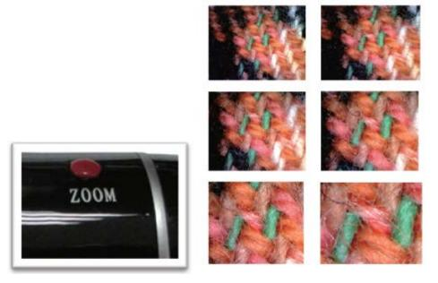
3. the final step is to press the "zoom" button, to do zooming: when you press "zoom" button one time, the object will magnified 1.3 times, press twice, it will magnified another 1.3 times, go on pressing until magnified the maximum, at this time if go on pressing, the image will resume the original size, you can process it circularly.
