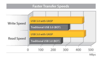
Note: UASP (USB Attached SCSI Protocol) is supported in Windows 8, 8.1, Server 2012 and Linux kernel 2.6.37 or later. Test results were obtained using an Intel® Ivy Bridge system, StarTech.com add-on USB 3.0 cards, a UASP-enabled StarTech.com enclosure, and a SATA III solid state drive.
